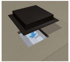
2 | Fixation of shuttering unit Level the shuttering units on the hollow floor before applying the screed.
