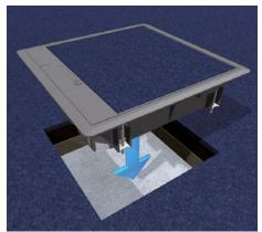
6 | Mounting assembly unit After the floor covering has been laid insert the installation unit straight into the opening and fasten it with the claws evenly to the screed.
