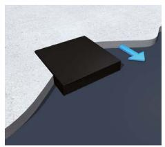
4 | Inserting screed Spread the screed on the whole area and compact it
